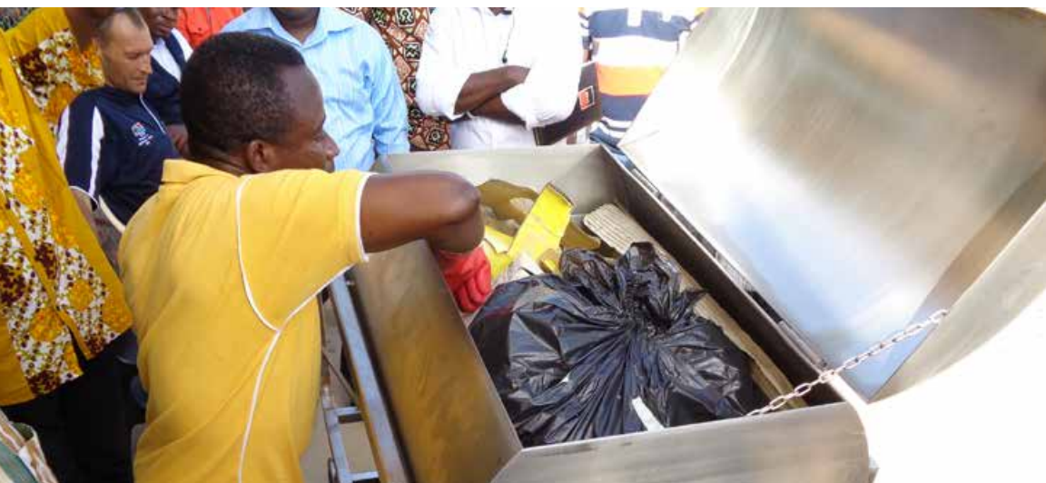
DEMONSTRATION OF THE USAGE OF AUTOCLAVES FOR WASTE TREATMENT IN GHANA. PHOTO BY JAN-GERD KÜHLING
