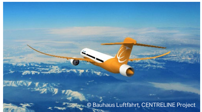
Figure 24: Propulsive Fuselage concept by Bauhaus Luftfahrt, integrating boundary layer ingestion and airframe wake filling
