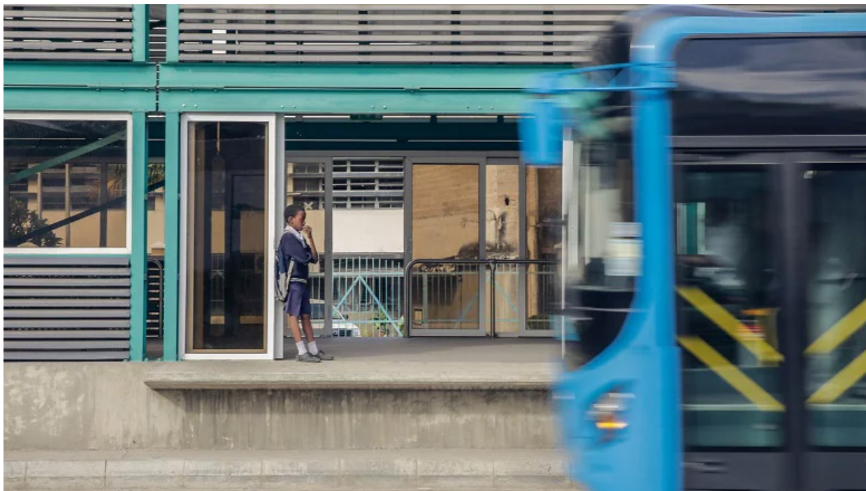
Figure 7. Level boarding at a BRT station in Dar es Salaam
